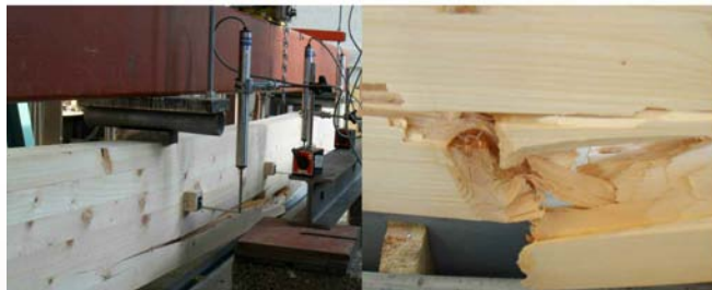
b) Sitka Spruce Failure
