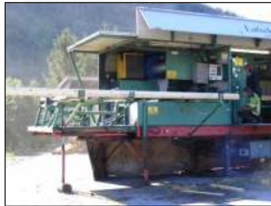
Solem Sag – mobile saw bench
