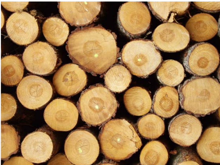
Figure 3: Scots pine sawlogs showing the relative proportions of heartwood and sapwood
