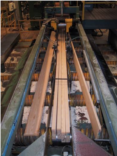
Primary breakdown (left) - a diverging process: one → many
