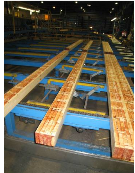
Gluing (right) – a converging process: many → one
