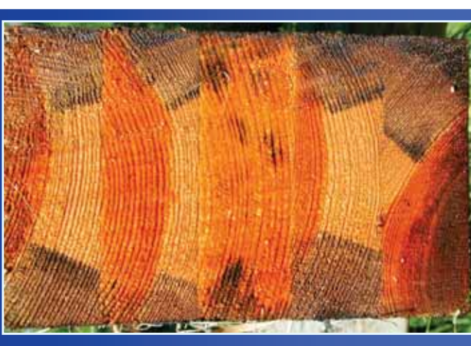
Cross section of pressure treated glulam
